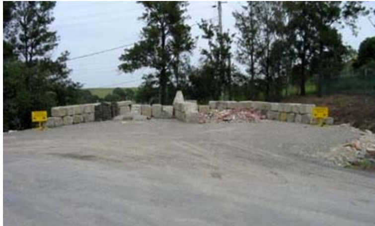
A dedicated unloading area for domestic C&D waste materials eliminates the risk of smaller vehicles coming into contact with larger trucks in restricted areas.
